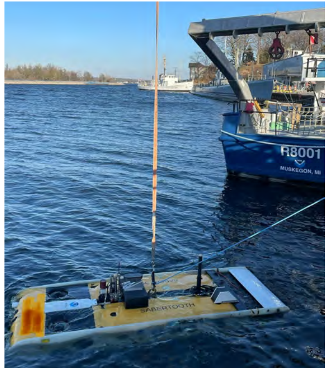
Testing deployments of an autonomous underwater vehicle in Lake Michigan, with the ultimate goal of using it under lake ice during winter to collect ecological and water quality data. Photo credit: Gabrielle Farina, NOAA Great Lakes Environmental Research Laboratory.
